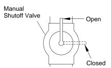
Figure 14 - Manual Shutoff Valve
